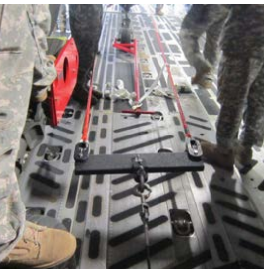
The HeliBasket Tow Bridle load testing an H-60 aboard a USAF C-17. Note the close proximity of the tow bridle and expected placement of the towed aircraft to the one to its left in the photo. (Photo: HeliBasket)
